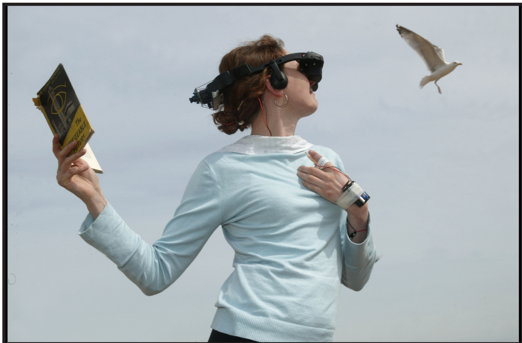
Sight unseen: Marieke Rohde is wearing a head-mounted display which gives her rear-view vision. The device relays images from a camera on the back of her head to miniature screens in front of her eyes. A vibrator on her index finger acts as an alarm. It warns her when she is getting too close to an obstacle. The vibrator is controlled by distance sensors attached to the front and rear of her torso
